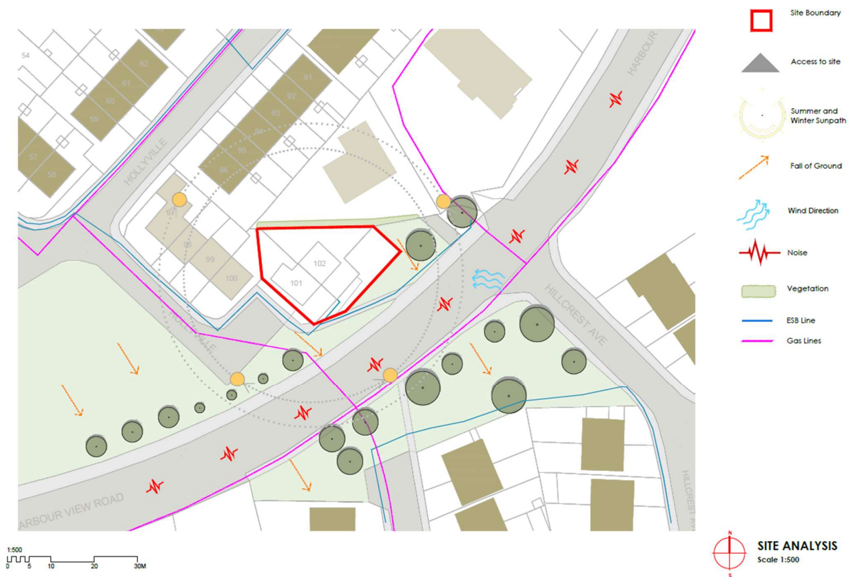
Fig. 6: Site analysis by author indicating prevailing wind, traffic noise, vegetation, services & fall of site and context.
